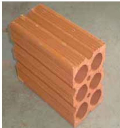
Fig. 1. Ceramic brick produced with sawage sludge (Herek and others, 2012).
