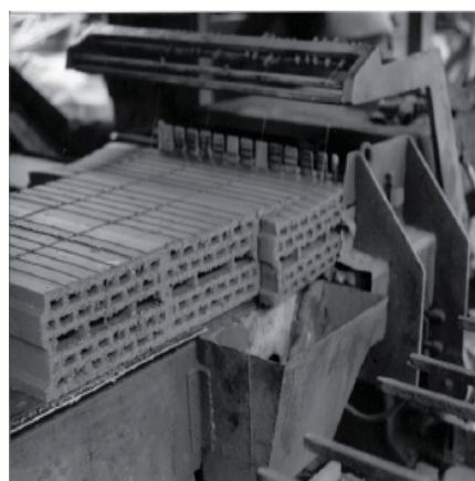
Fig. 2. The industrial production of the ceramic materials made of clay, sewage sludge and forest waste (Devant and others, 2011).
