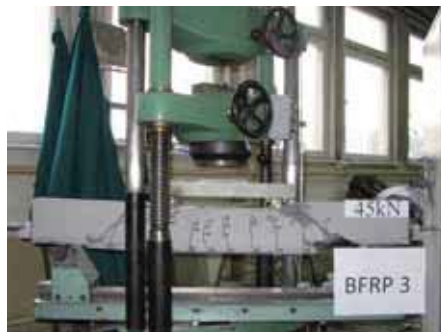
Fig. 3. The BFRP beam with flexural basalt reinforcement reaching critical load capacity equal to 45 kN (Lapko and Urbanski 2013)
