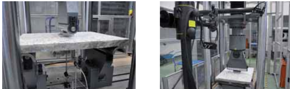
Fig. 1. Laboratory stand for testing reinforced concrete plates.
