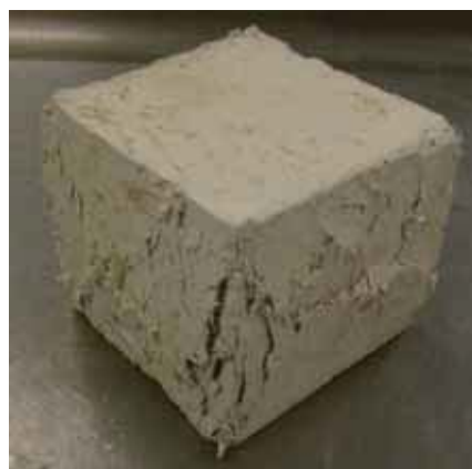
Fot 9. Destroyed sample after the compressive strength test
