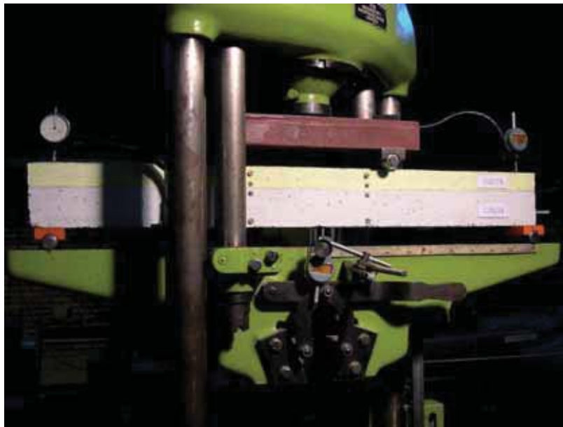
Fig. 2. The beam on the test stand in the testing machine.(Sadowska-Buraczewska,2012)
