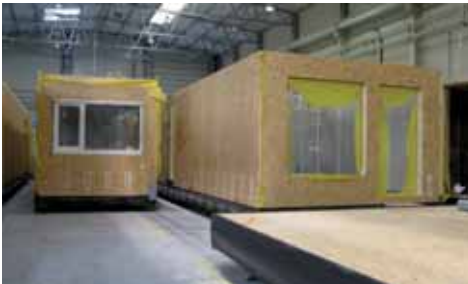
Fig. 8. Stages of module assembling: a) sub-assembly of floor elements, production of wall panels, c) assembling of module structure (UNIBEP)
