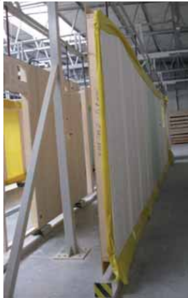
Fig. 8. Stages of module assembling: a) sub-assembly of floor elements, production of wall panels, c) assembling of module structure (UNIBEP)
