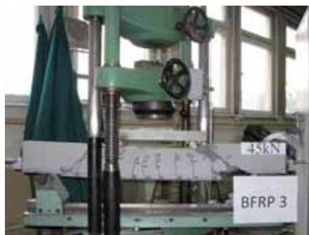
Fig. 3. The BFRP beam with flexural basalt reinforcement reaching critical load capacity equal to 45 kN (Lapko and Urbanski 2013)
