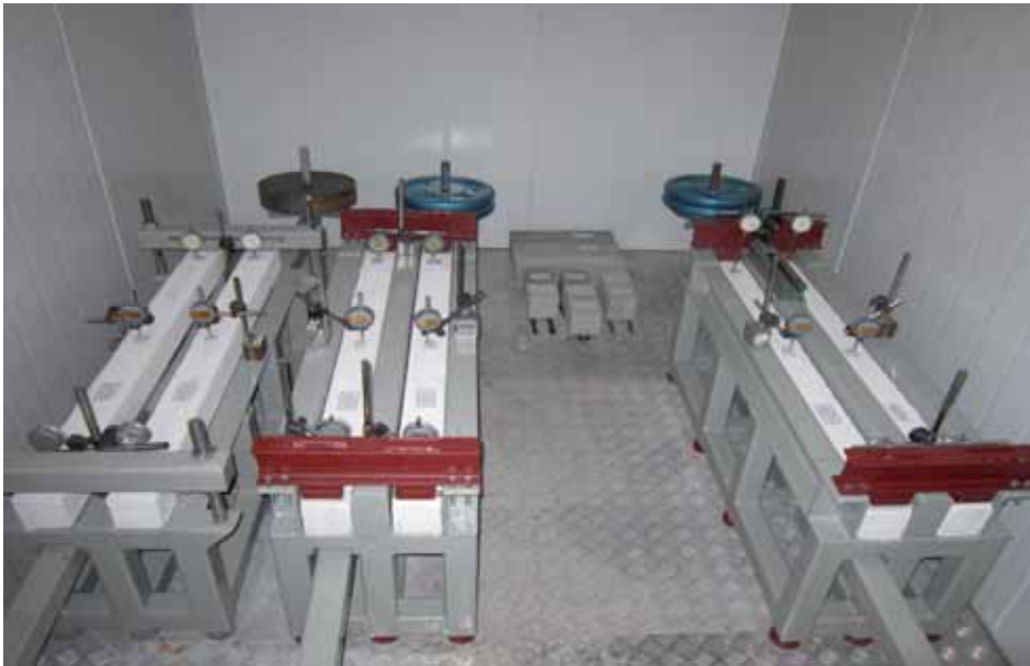
Fig. 5. The research stands with the model RC beams in the climatic room during the tests
