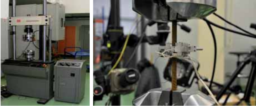
Fig. 2. MTS 810 material test system and steel bar during the axial tensile test
