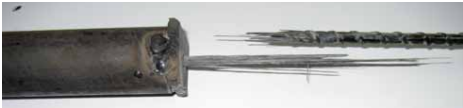
Fig. 1. Failure mode of the rupture of basalt bar (Urbanski et al 2013)
