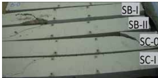
Fig. 6 The failure modes of selected SFRC beams after testing (Iwaniuk, 2012)
